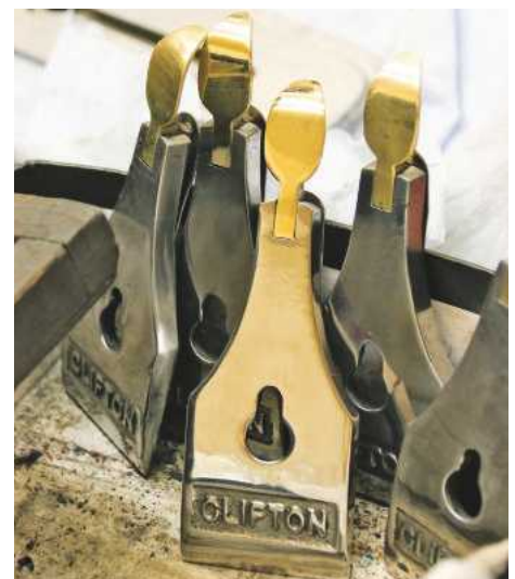
▲ These lever caps show the high polish achieved before they leave the factory
